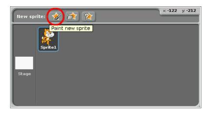
This displays a **paint editor** that can be used to create a new sprite of your design. The other buttons to the right allow saved sprites to be loaded (Scratch comes with many different sprites) and a random sprite to be added to the sprite list.
