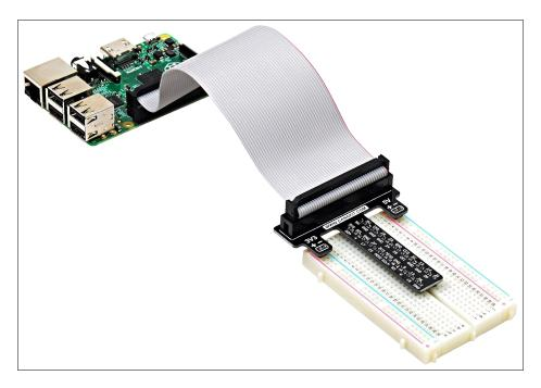
It extends the RPi's GPIO pins to the breadboard, making it easier to prototype circuits. For example, LEDs, resistors, and other electronic components can be easily placed on the breadboard. Typically, the breadboard will be provided with power from the RPi through several GPIO pins. Sometimes, we may use input devices (such as push-button switches) that can be *read* by the RPi by our computer programs.
