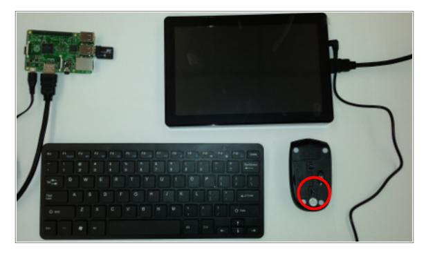
Finally, plug the power adapters into electrical outlets. This will turn on the Raspberry Pi and the LCD touchscreen. The system will quickly boot to an installation mode:
